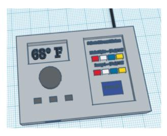
The second model was also created using TinkerCAD, and built on the preliminary with defined dimensions, curved edges, and a thinner design. The dimensions of this model were used to determine the final dimensions of the product.
